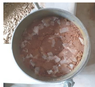
Figure 5. Penetration Occurred in Reinforced Soil Sample after CBR TEST
