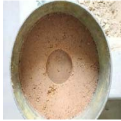
Figure 6. Penetration Occurred in Unreinforced Soil Sample after CBR TEST
